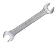
The open-end spanner is forged from chromium-vanadium steel. Surface protection chrome plated, polished head. The open-end spanner is used for tightening, loosening bolts, nuts and other fasteners. Place the open-end head on the bolt or nut, then turn the spanner clockwise to tighten or counterclockwise to loosen the fastener. When doing this, make sure that the open-end head fits correctly on the fastener to prevent damage or slippage.
