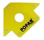
Magnetic square for angle welding, 135, 90 and 45-degree angles. The maximum load capacity is 33kg. 6 different angle placements are possible. Ideal for holding materials during welding and brazing. The hole in the centre of the square allows for easier removal after work.
