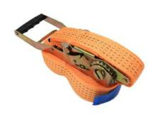
Strapping is a broad term referring to different types of straps and bands used to tie, tighten, hold or fasten various objects. Strapping made of durable material, usually nylon or polyester webbing and duck webbing, is used to secure and tighten loads on vehicles. Load capacity up to 5 tones.
