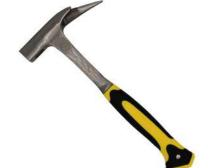
A highly durable one-pcs roofing hammer made of high-quality carbon steel. The head is polished and contains a magnet, allowing one-handed use. The handle of the hammer is made of fibreglass and is additionally coated with rubber for a comfortable and secure grip.
