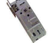
Lock for wooden doors up to 60kg. Suitable for both interior and exterior doors. The lock is universal, which means it is suitable for both left and right-hand doors. The lock is made of steel and zinc-plated to protect it against corrosion. It is double-locked, made in accordance with the JUS and certified for 200,000 openings/closings. The lock is made for a standard key.
