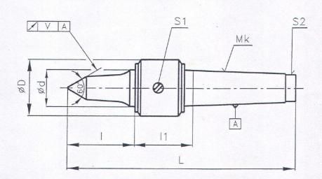
The centres are intended for the clamping of workpieces on NC lathes. Their clamping part allows for on easy access of the tool to the workpiece, which is particularly advantageous during machining of form workpieces. The desing allows for the adjustability of the clearance in the radial bearing. The live centre is provided with the shank with Morse taper according to CSN 2204208 (DIN 228, ISO296) without the clamping thread.
